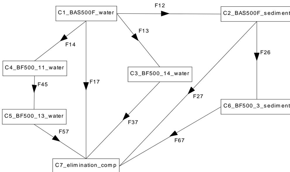
The coefficient of determination for the whole model was  $r^2 = 0.994$ . The half-lives of pyraclostrobin and metabolites are shown in Table B.8.4-17. For the metabolite BF 500-13, no reasonable half-life could be calculated in this study, however, the results of the aqueous photolysis study (LUF2000-249) clearly showed that also this metabolite is degradable in water under irradiated conditions.
